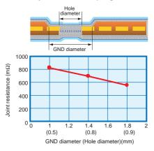
Fig. 8 Ground joint resistance (Double-sided shielding)
