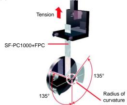
Table 2 MIT flexural endurance test conditions
