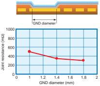
Fig. 7 Ground joint resistance (Single-sided shielding)
