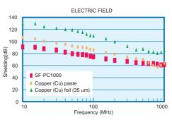
Fig. 6 Shielding characteristics (KEC method)
